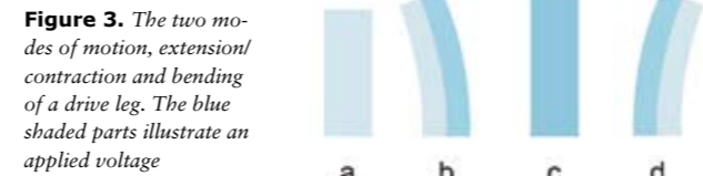
Figure 3. The two modes of motion, extension/contraction and bending of a drive leg. The blue shaded parts illustrate an applied voltage
